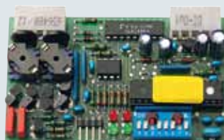
Induction loop detector 1 or 2-channel plug-in print suitable for two separate induction loops, supplied without loop cable
